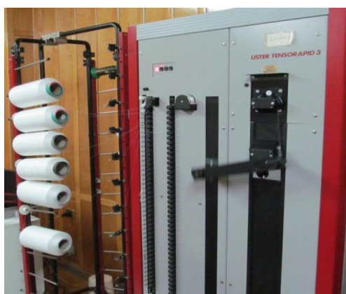
Figure 2. Automatic multiple tensile test
